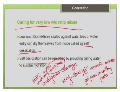
That is what I told you for very low water to cement ratio mixes let us say lesser than 0.35. So, 0.3 for very low water cement ratio for high strength concrete mixes it is preferable to go for curing by external application of water. So, that will be the best method. Because what happens is if you go for methods like which just prevents the loss of water from within concrete to outside environment.
