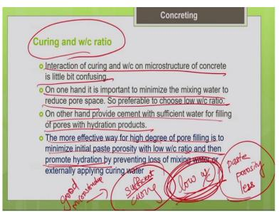
Because on one hand we say that we need sufficient water for the complete physical and the chemical hydration of the cement. On the other hand, we say that when we add excess water, it leads to high paste porosity that will affect the microstructure strength and the durability. So, then what is the best measure to get a good microstructure? So, what is the best solution? So, the best thing is you always go for low water to cement ratio.
