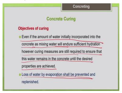
So, even if the amount of water initially incorporated into the concrete as mixing water will endure sufficient hydration. However, curing measures are still required to ensure that this water remains in the concrete until the desired properties are achieved. So, even though the water which you have added for concrete making is sufficient, even then you have to do curing so that you can prevent the loss of this water to the outside environment.
