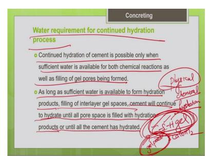
As I just mentioned now, so, for the hydration process to continue, we need water. So, the hydration process occurs in different forms, physical hydration, chemical hydration. So, chemical hydration everyone will be knowing. So, chemical hydration is nothing but the water needed for the reaction of your cement compounds with the water to form the hydration products, so, silicates and the aluminates.
