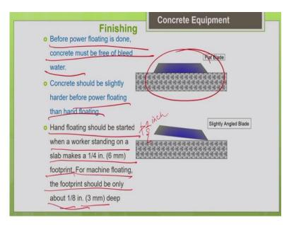
So, the important guidelines you should keep in mind is, so, generally the window of the finishing period is between the initial set and final set. So, the concrete should have dried up well and it should be free of bleed water. So, then only you should do the finishing operation. Particularly when you are going to use your machines as I told you the concrete should be able to withstand the weight of the machine.
